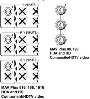
Figure 2-13 — MAV Plus component/HDTV video connections
